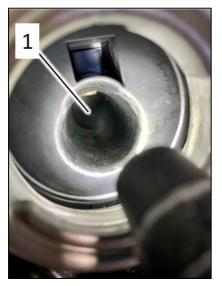
Fuel condensation formed on adapter cap <1>.
