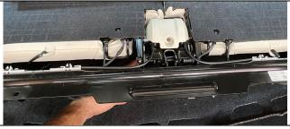
You can feel the springs easier than you can see them. Here we are pointing at the Left Hand Inboard (LH IB) compression spring.
