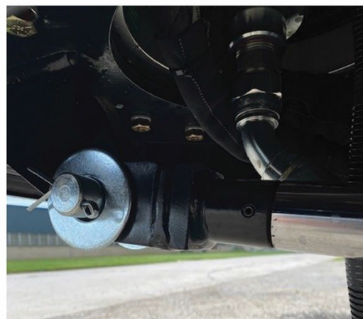
Image showing updated clevis installed
