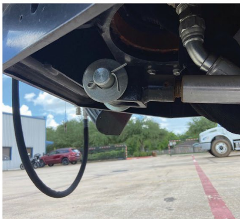
Image showing original clevis installed
