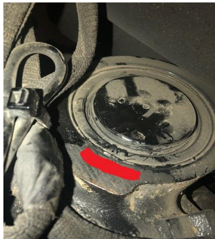
Figure 1: Serial Number and Part Number Location (Red Field is Example of Location)
