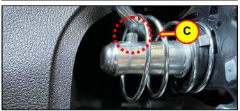
Use an H4/H5 Allen wrench/screwdriver to depress the airbag fastening pins.
