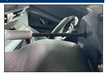
Insert the Allen wrench/screwdriver until it cannot go in any further. Gently press the end of the Allen wrench/screwdriver upward to depress the pin.
