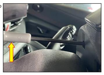
5B. To release the bottom fastening pin, insert the Allen wrench/screwdriver and push inward to depress the pin.
