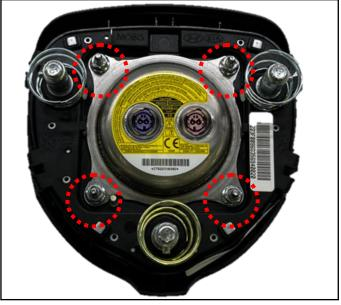
3. Separate the driver airbag cover from the airbag inflator module.
