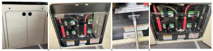
2) Remove the upper black panel by removing the 5 Phillips screws and flexing it out of the opening.
