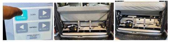
3) Remove the top black plastic cover panel on the battery box. This panel has Velcro on the back edge. Lift the cover and slide it out. This will give you access to the DCD panel. Locate the two fuse holders on the DCF4 board.
