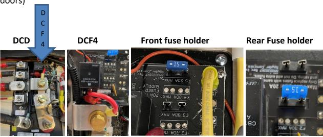
5) Remove the paper back on the label. Place the label around the rear fuse holder. The fuse label will be installed with the writing between the front and rear fuses holder. The writing will be upside down when reading it from the rear doors.
