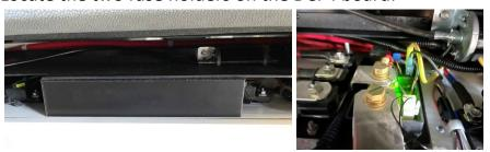
4) The DCF4 board is located towards the front of the DCD panel on the right hand side. A 15 amp fuse will be located in the front or rear fuse holder. (As viewed from the rear doors)
