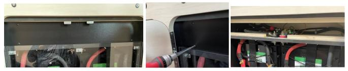
3) The DCF4 board is located closest to the passenger side outer wall on the right hand side of the DCD. Front and Rear fuse holder will be on the DCF4 board, currently there are no fuses in these holders as this portion of the circuit board is not used for OEM operation.
