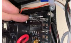
5) Reinstall the black cover panel with the Phillips screws removed in step #2 and slide the Plexiglass panel up and lock it back into place that was removed in step #1.
