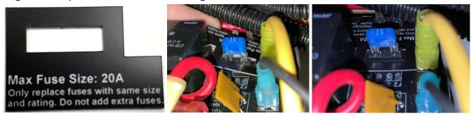
6) Replace the black cover panel. Ensure the black sofa cable is above the panel and all other wiring is below the panel.
