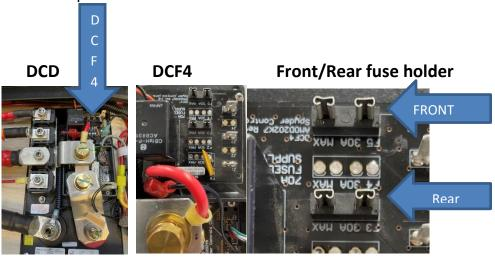
4) Remove the paper back on the label. Place the label around the rear fuse holder. The fuse label will be installed with the writing between the front and rear fuses holder. The writing will be upside down when reading it from the cabinet doors.
