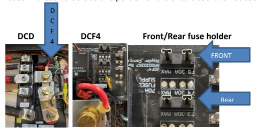
4) Remove the paper back on the label. Place the label around the rear fuse holder. The fuse label will be installed with the writing between the front and rear fuses holder. The writing will be upside down when reading it from the rear doors.
