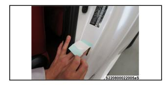
b) Remove the release paper from the upper side of the **NEW** label as shown in the illustration, and apply the label.
