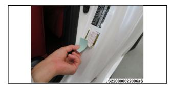
c) Remove the release paper from the lower side of the label, and apply the label.
