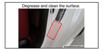
b) After removal, degrease and clean the vehicle surface thoroughly.
