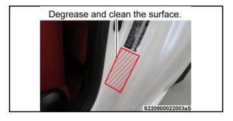
b) After removal, degrease and clean the vehicle surface thoroughly.
