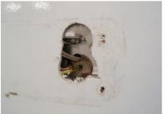
B. YOU MAY HAVE TO USE A TOOL TO REMOVE SOME OF THE ALUMINUM TUBING TO ALLOW SPACE FOR THE WIRING ON THE BACK SIDE OF THE NEW TAIL LAMP;
