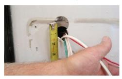
G. DRILL 3/4" HOLE BELOW THE TAIL LAMP HOLE A MINIMUM OF 2";
