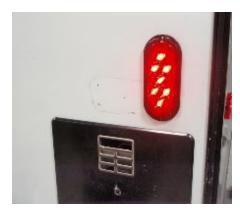
E. INSTALL COSMETIC SNAP RING FOR NEW TAIL LAMP AND CAP SEAL WITH SILICONE.
