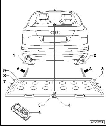
After rear lid is replaced, calibrate the rearview camera. See ELSA Repair Manual: Repair manual > Electrical System > Communication > 91 Communication > Rearview Camera System > Rearview Camera System, Calibrating
