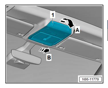
• Pry out the roof module <1> in the rear area in the direction of <arrow A> using a commercially available plastic wedge.
