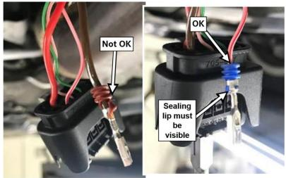
Figure 4 ( not OK and OK sealing element)
