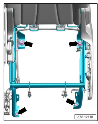
• Release the hooks <arrows> and remove the trim panel forward.
