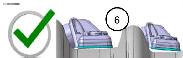
**NOTE:** Installation OK, positioning of wheel electronics module on rear edge in rim well base (6).
