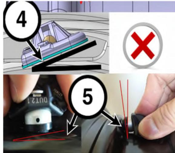
**NOTE:** Installation OK, flat/parallel positioning of the wheel electronics module on rim well base(6).
