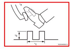
Depress the brake pedal to full stroke, two times within two seconds before reprogramming. This will prevent the brake booster pump from starting during reprograming which could result in a voltage drop. <u>Do</u> <u>not</u> depress the brake pedal again until reprograming is completed to prevent voltage drop.
