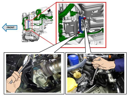
**TIP 3)** It is not necessary to remove the entire PCV pipe. Detach the pipe from the holding clamp. This will avoid replacement of the PCV pipe which is a one-time use part.
