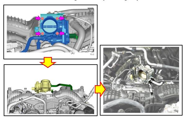
**TIP 5) CAREFULLY** raise the vehicle and disconnect the five electrical connectors and the harness mounting clips. Remove the mounting bolt and the spring lock on the intake duct. Refer to the images below.
