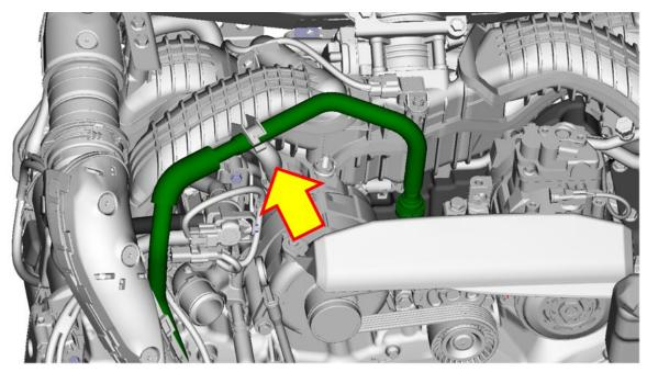
**TIP 4)** The throttle body assembly does not have to be fully removed. Remove the four mounting bolts and disconnect the wiring harness connection. The throttle body assembly can be repositioned with the pre-heater (coolant) hoses attached to gain sufficient access. Use CAUTION to not damage the throttle plate during this procedure.
