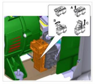
4. Wait for more than 5 minutes so that the capacitor in the high voltage system can be fully discharged.
