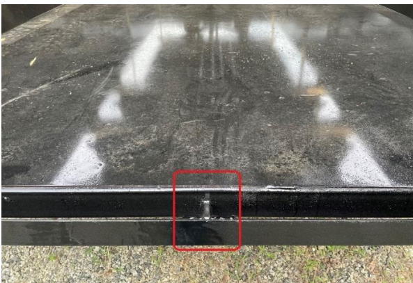
Properly Installed Angle Ramp Track with Caps, Gussets and Welds
