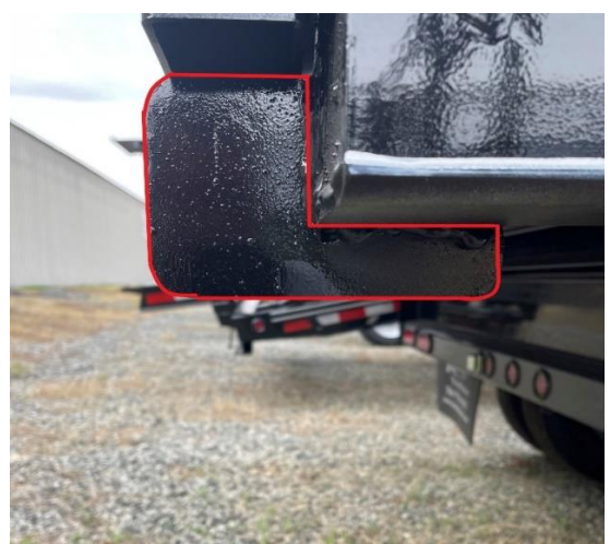
Center Gusset on Angle Ramp Track Installed
