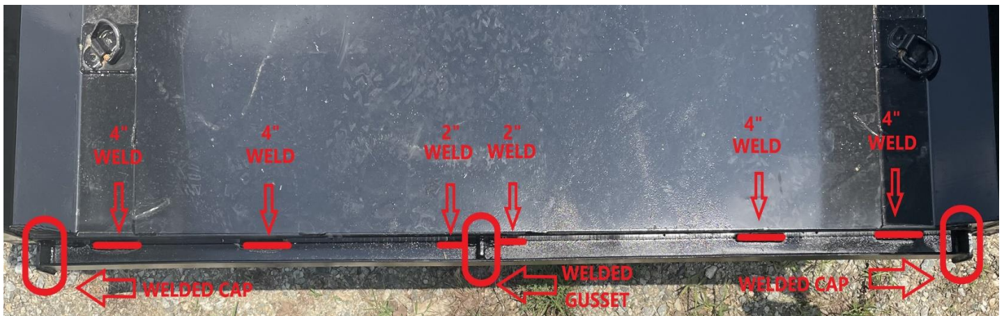
Properly Installed Angle Ramp Track with Caps, Gussets and Welds
