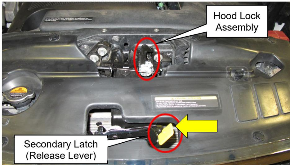
Figure 1 – Hood Lock Assembly and Secondary Latch
