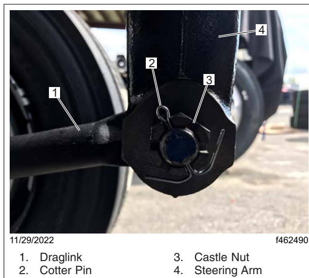
Fig. 5, Cotter Pin Removal
