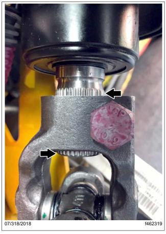
Fig. 2, Steering Shaft Splines
