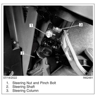
Fig. 1, Steering Pinch Bolt Location
