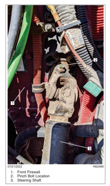
Fig. 4, Pinch Bolt and Front Firewall Location
