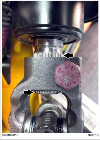
Fig. 2, Steering Shaft Splines
