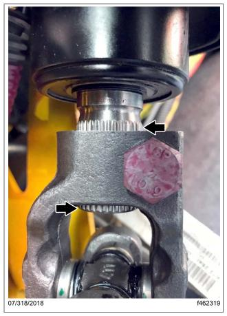
Fig. 2, Steering Shaft Splines
