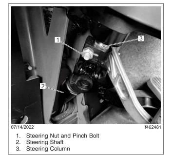
Fig. 1, Steering Pinch Bolt Location
