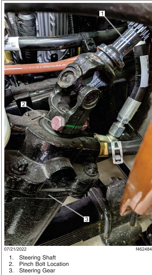
Fig. 5, Pinch Bolt and Steering Gear Location
