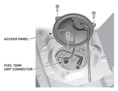
3.4. Disconnect the fuel tank unit connector.
