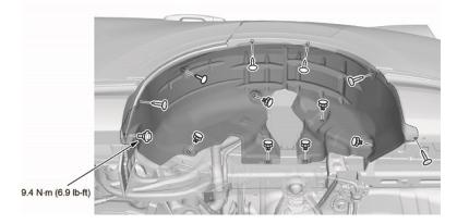
7. Remove the heat shield from the right rear area.
