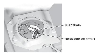
3.6. Unlock the fuel tank unit cam lock ring.
