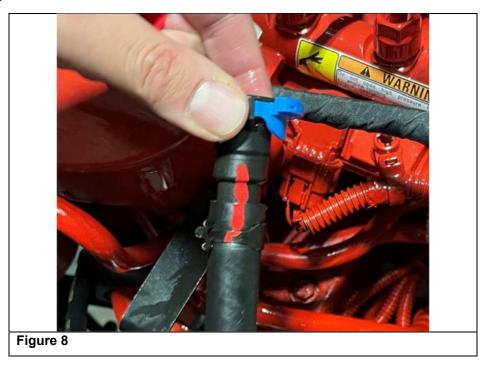
12. Push the new fitting onto the engine and listen for a "click". Push the blue lock tab towards the fitting until it is in the locked position. (See Figures 9 and 10.)
