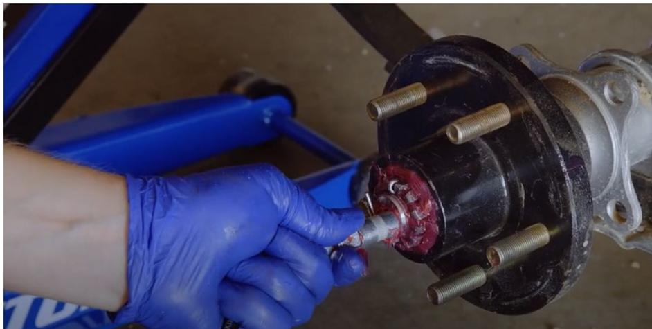
13. Reinstall the cap removed in step 4.
