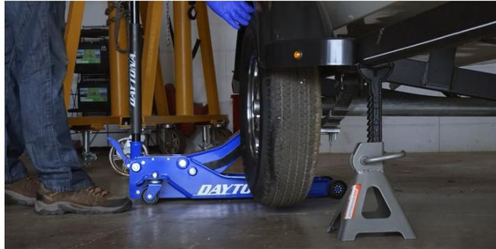
2. If 18-inch wheels are installed on the trailer, remove the wheel. All others, service can be done with wheels installed.
