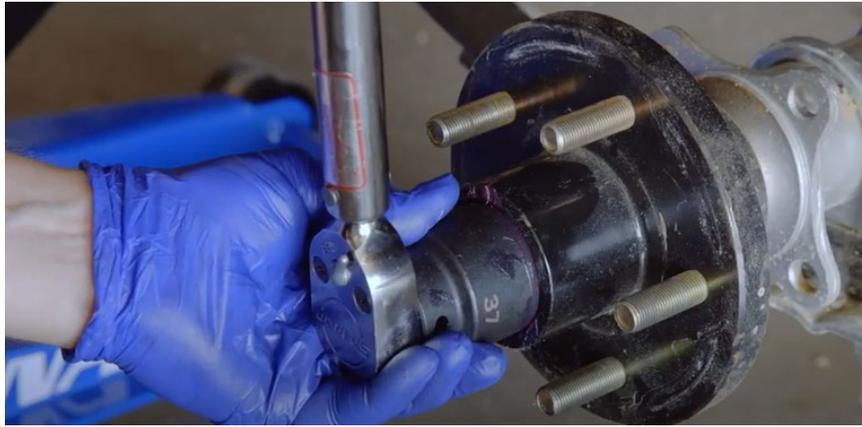
8. Loosen the castle nut to remove the torque applied. DO NOT ROTATE THE HUB.
