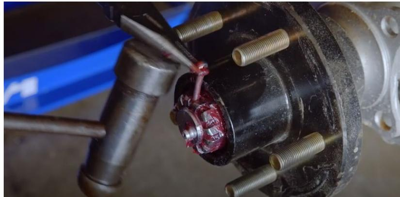
7. Apply 50 ft. lbs. of torque to the 27 mm castle nut. This “seats” the bearings.
