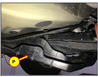
10. Release the low-pressure fuel line from the bundle clip (Q).
