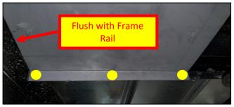
4. Align the top of the heat shield with the top of the mounting tube. Secure with (3) TEK screws. (Fig. 3)
