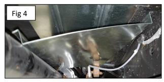
6. Align the edge of the heat shield with the chassis frame rail. Secure into angle with (4) TEK screws on each side flange. (Fig. 5)
