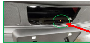
Figure 2 1 Radar Not Installed
