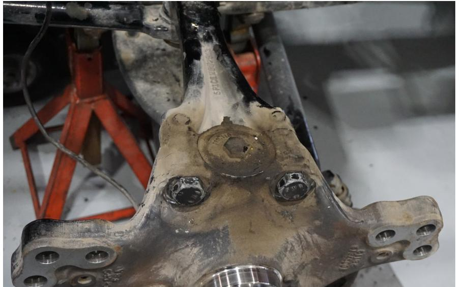
**Step 12:** Clean spindle for reinstallation.
