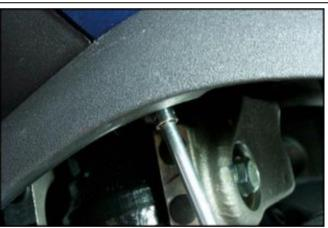
Remove both front mudguards, pushing towards the front of the vehicle to detach all the fastener lugs.
