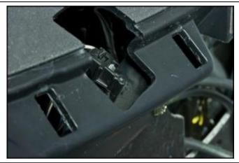
Remove the 2 rear fastener screws of the dashboard.
