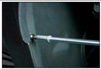
Remove the upper fastener screw of both mudguards.
