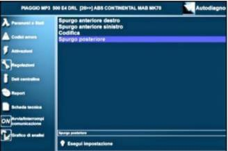
Before accessing the activation of the modulator, the message intended to prevent any unaware use of the modulator bleeding phase is displayed.
