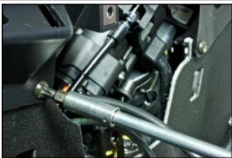
Using a pair of circlip pliers, turn the bezel of the ignition switch anticlockwise to align the word 'ON' with the key slot.
