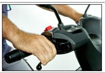
At the same time, press the combined braking system master cylinder pedal.
