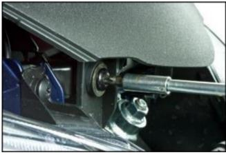
Remove the windscreen mount, removing the remaining 4 fastener screws with the relative shaped spacers.
