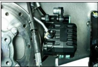
Pull the rear brake lever repeatedly to bring the brake pads into contact with each other.
