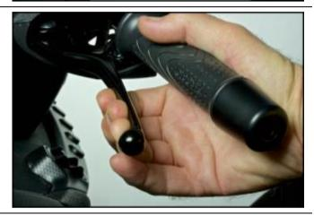
When the pressure of the electric pump prevails over the manual pump, maintain the pressure by reducing the stroke of the lever as necessary.
