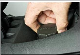
Remove the centre cover, detaching the cable for internal saddle sensor and the fuel filler cover release cable.
