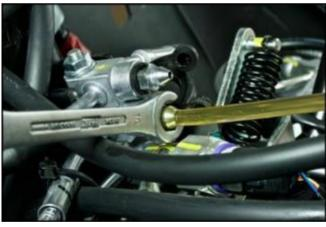
Remove the upper fasteners of both front callipers and restrain the callipers temporarily in a vertical position.
