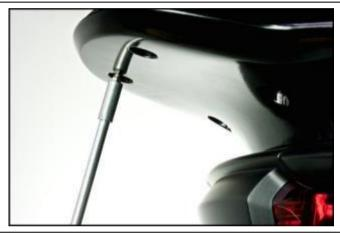
Use a screwdriver to prise out the 2 blanking plugs of the holes for the 2 front fastener screws of the grab handle.
