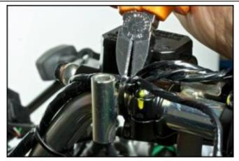
Adjust the fastener screws of the handlebar clamp U-bolt to bring the brake fluid reservoir as close as possible to the horizontal position.
