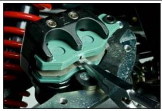
Provisionally fit the callipers onto the rear disc. Operate the rear master cylinder to set take up the clearance between the pads and the disc.
