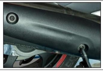
Loosen the screw of the metal clamp fastening the silencer to the exhaust pipe.
