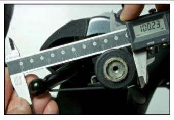
N.B: The measurement must be made with the vernier calliper perfectly aligned with the direction of movement of the lever.
