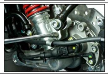
Remove the lower fastener screw of the left hand calliper and separate the pads, pushing the pistons to their respective end stops.
