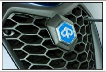
Remove the Y-shaped cover, detach the respective fastener lugs.
