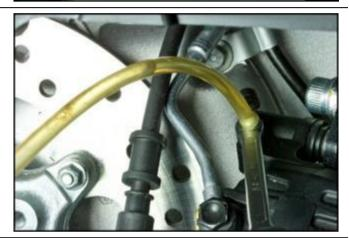
Pull the lever to operate the master cylinder and repeat the bleed sequence while observing the fluid drained from the calliper bleed nipple to check for air bubbles.
