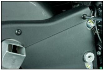
Remove the speed sensor, unscrewing the 2 fastener screws.
