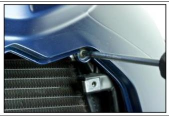
Remove the front cover, unscrewing the 2 Torx screws.
