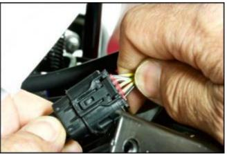
Release the lock tab and disconnect the dashboard connector.
