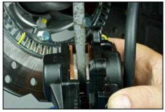
Hold the right hand calliper in a vertical position and pressurise the master cylinder.
