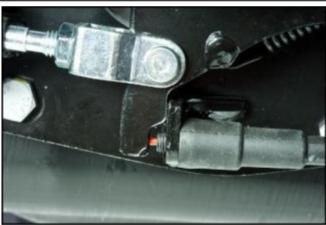
Press the pedal to release the brake light switch and reveal the clearance created between the **pedal arm** and the actuator pin of the brake light switch
