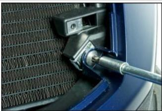
Remove the 2 upper screws fastening the bodywork mount.
