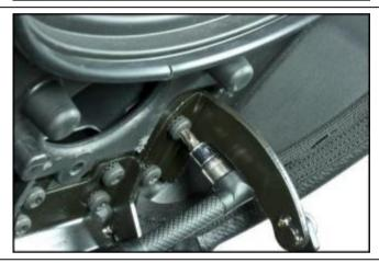
Remove the fastener screw and the cover of the internal saddle sensor.
