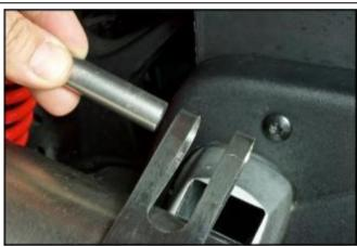
Remove the mounting screw of the silencer with the relative washers, and detach and remove the silencer from the exhaust pipe.
