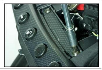
Release the 2 clips and disconnect the button panel, disconnecting the 4 electrical connectors.
