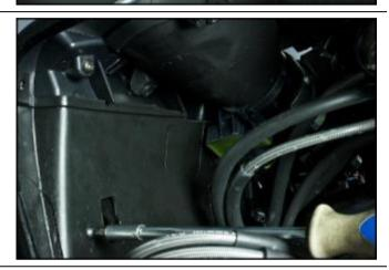
Remove the fastener screw of the expansion tank cap access cover.
