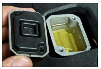
Operate the rear brake lever repeatedly. Keep the master cylinder under pressure.
