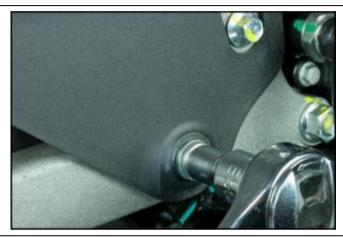
Remove the plastic guard panel, unscrewing the remaining 2 upper screws.
