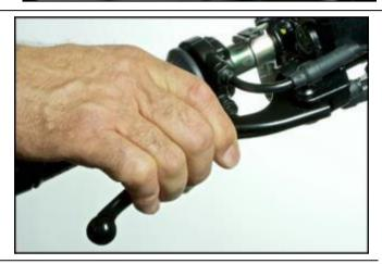
Pull the front brake lever and hold in position by fitting the O-ring, p/n 006731, onto the lever and handgrip as shown in the photo.
