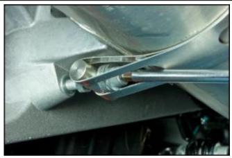
Remove the pin and remove the retainer bracket.
