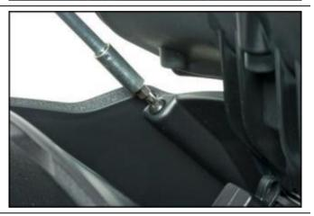
Remove the 2 front fastener screws of the windscreen mount complete with the relative washers.
