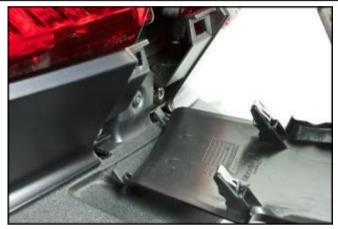
Remove the lower screws of both side covers.
