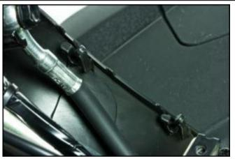
Disconnect the connector of the ambient temperature sensor.
