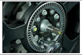
Continue with the reassembly of the carrier arm, paying attention to the correct application of all the tightening torques.
