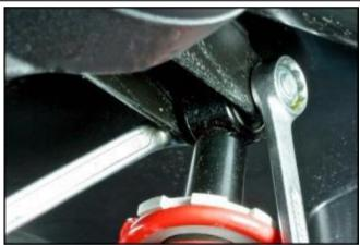
Remove the right hand shock absorber with the 4 spacers.
