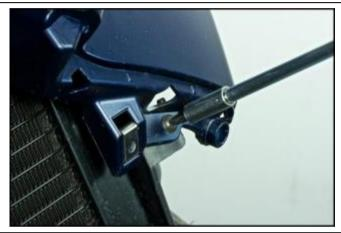
Remove the 2 upper fastener screws of the leg shield.
