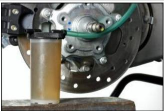
Fill the rear master cylinder reservoir to the max. level.
