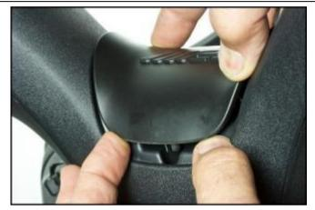
Remove the fastener screws and disconnect and remove the handlebar switchgear sets.
