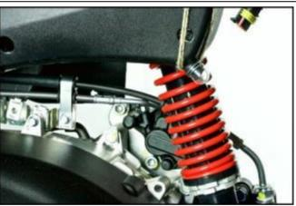
Use a screwdriver to straighten the anti-rotation tabs of the fastener screws of the calliper mounting bracket.
