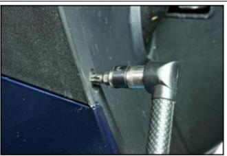
Remove the lower fastener screw of the right hand footboard.
