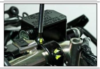
Hold the rear brake master cylinder in a vertical position.
