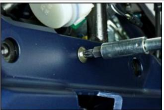
Remove the front leg shield, unscrewing the remaining 4 fastener screws.
