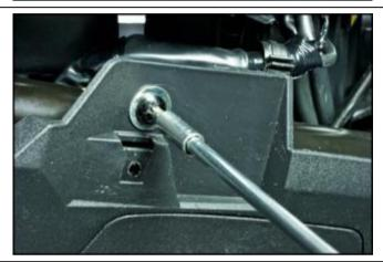
Remove the right hand rear footrest platform, unscrewing the clamp screw and unscrewing and removing the 2 Torx screws complete with the relative washers.
