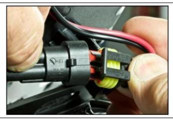
Release the lock tab and disconnect the flying lead connector of the dashboard connector.
