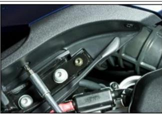
Remove the 2 screws fastening the centre cover, near the saddle.
