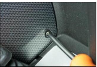
Remove the 2 fastener screws of the right hand centre cover.
