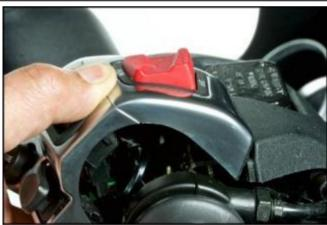
Remove the fastener screws of the handlebar cover, situated in the space under the handlebar switchgear sets
