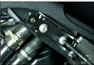
Remove the 4 screws connecting the underside of the footboard to the footboard.
