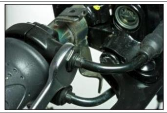
Remove the 2 screws and the handlebar clamp Ubolt of the right hand master cylinder.
