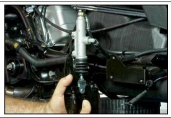
Connect the fluid collector container to the bleed nipple of the front brake servo pump and pump the pedal a few times while checking for air bubbles in the drained fluid.
