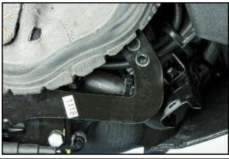
Bleed the front brake servo pump until the fluid drained contains no more air bubbles.
