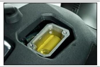
Continue filling the rear brake circuit until approximately 120 cc has been drained into the collector container.
