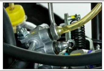
Repeat the step to check if the fluid drained from the upper bleed nipple of the right hand circuit contains air bubbles.
