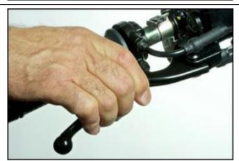
If the ABS modulator had air inside, this would have transferred into the lines between the ABS unit and the front callipers, restore them by bleeding from the fittings of the upper branches.
