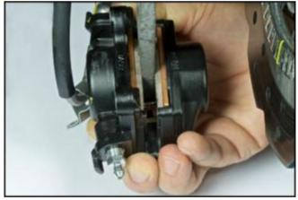
Hold the left hand calliper in a vertical position and pressurise the master cylinder.
