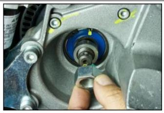
Remove the lower fastener bolt of the shock absorber.
