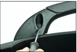
Remove the rear grab handle, undoing and removing the 5 screws with the relative washers.
