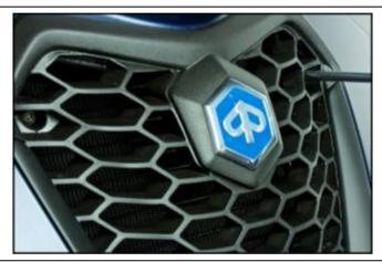
Remove the front fastener screw of the 2 mudguard.
