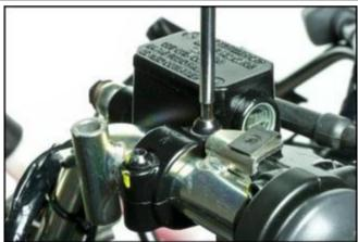
Rotate the right hand master cylinder into a vertical position.
