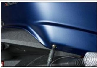
On both flanks, remove the 2 screws near the passenger footpegs.
