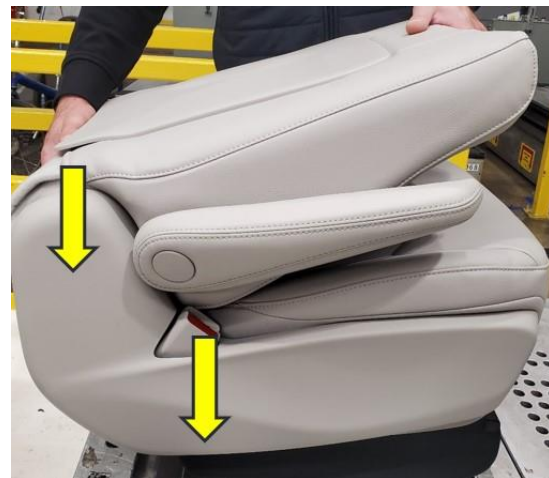
Figure 6 – Latch Seat to Floor
