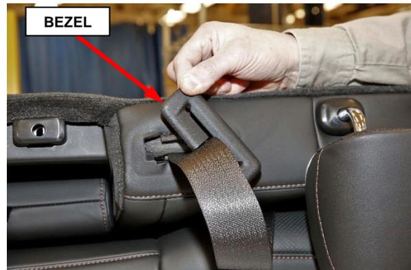
**Figure 29 – Center Seatbelt Bezel**
