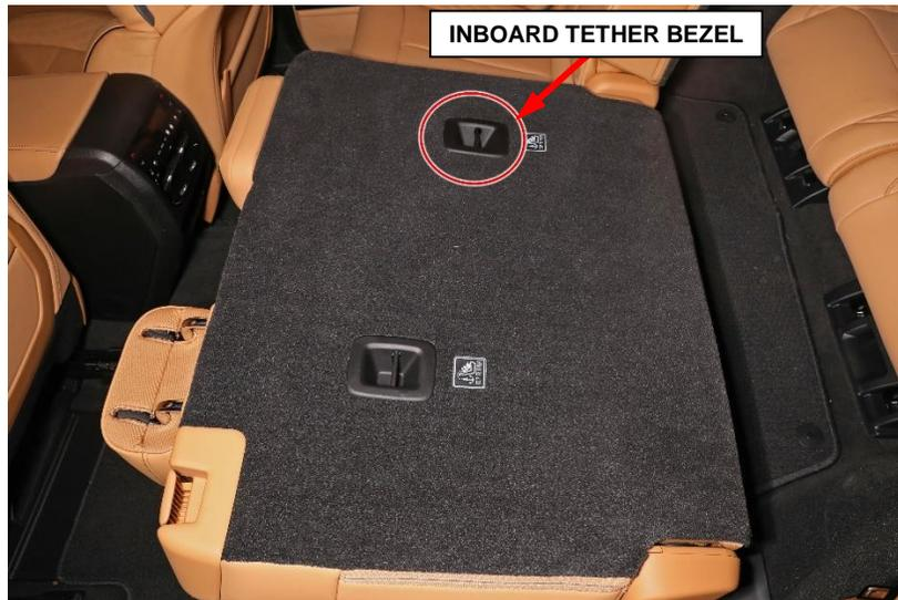
**Figure 8 – Split Bench Seat 60% Side Inboard Tether Bezel**
