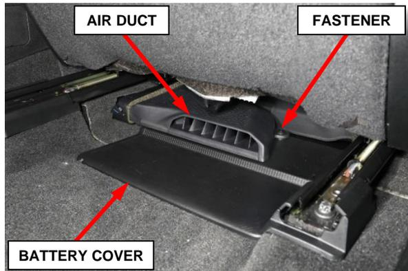
**Figure 70 – Air Duct and Battery Cover**
