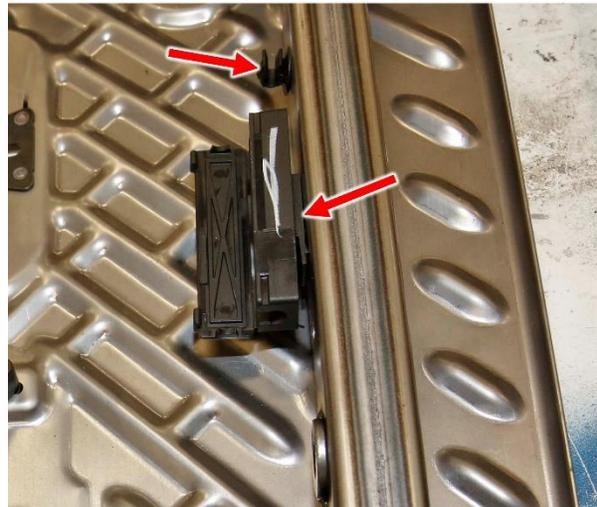
**Figure 40 – Headrest Cable Retainer and Junction Box**
