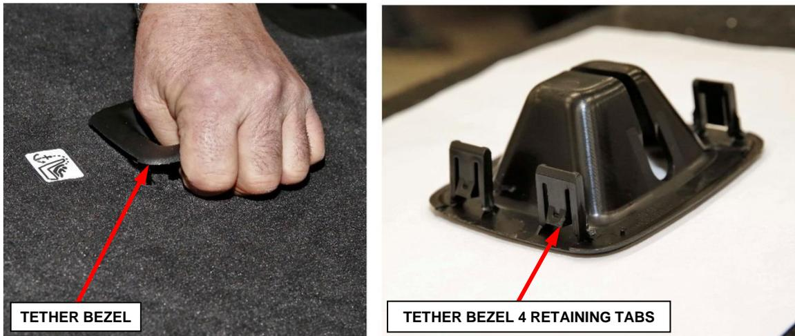
**Figure 7 – Tether Bezel 4 Retaining Tabs**
