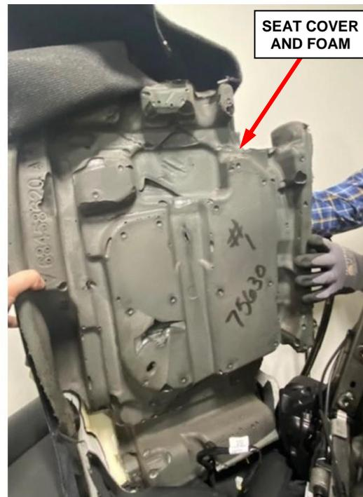
**Figure 81 – Seat Cover and Foam Assembly**
