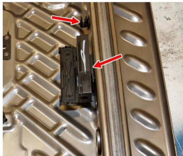
**Figure 66 – Headrest Cable Retainer and Junction Box**
