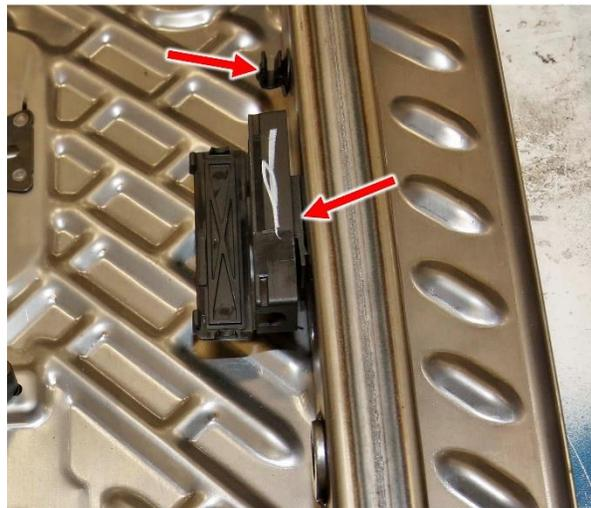
**Figure 89 – Headrest Cable Retainer and Junction Box**
