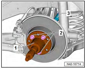
Attach Drive Shaft Remover Kit -T10520A to the wheel hub using three wheel bolts
