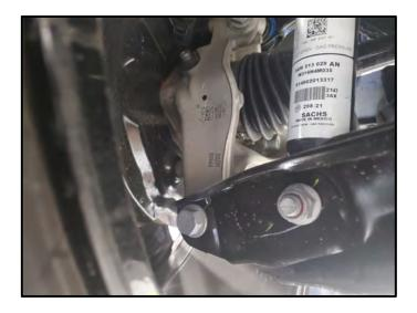
Inspect rear wheel bearing housings and replace, if necessary.
