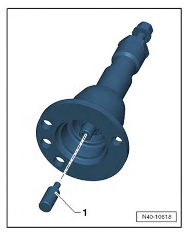
If the drive axle cannot be pulled out of the wheel bearing, then the drive axle can be pushed out of the wheel bearing using the Drive Shaft Remover -T10520A-.
