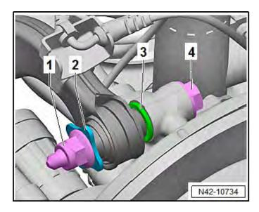
• Counter-hold bolt <4> and torque nut <1> to 130 Nm + 180° in curb weight position.
