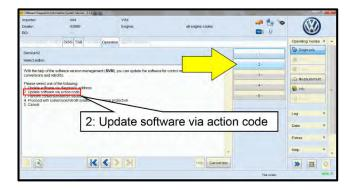
Once the GFF scan is complete, select "Special functions" <arrow 1>, then "Adapting software" <arrow 2>, then select "Perform test" <arrow 3>.
