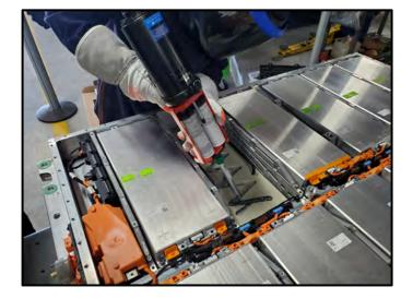
• Clean the bottom of the cell module using Cleaner D -009-401-04 or isopropyl alcohol and allow it to dry completely.
