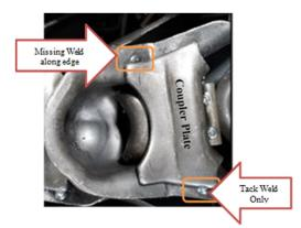
To Fail Inspection: A weld bead will not run along the side of the plate and there will only be tack welds
