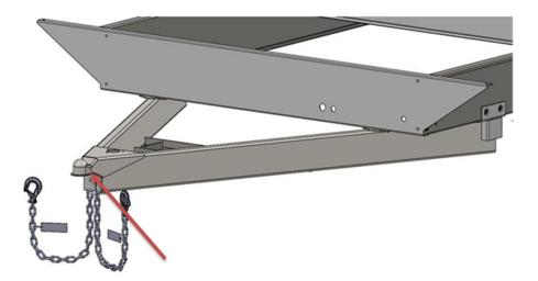
2. Underneath the coupler, use a flashlight to inspect the welds at each side of the bottom coupler plate.
