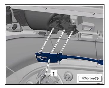
Disconnect the cable <1> from the interior door mechanism.
