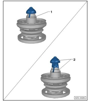
• Disconnect the cable <1> from the interior door mechanism.
