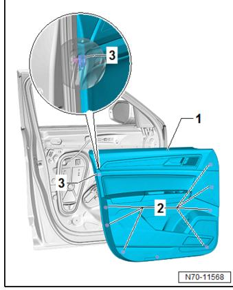
• Turn/release the rotor clip <1> 90° in the <direction of the arrow> (1/4 of a turn) using the open end wrench (10 mm) or Torx T30.
