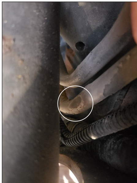
Figure 11 — Fuel Line Replacement-Level Damage Example— REPLACEMENT REQUIRED
