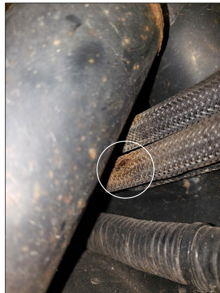
Figure 12 — Fuel Line Cosmetic Damage Example— Replacement Not Needed
