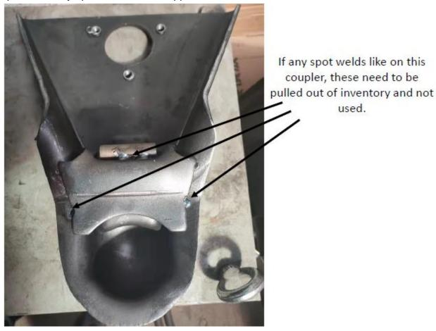
If the coupler appears to be spot-welded only, the trailer should not be towed. The coupler must be replaced where it is located. If this situation exists, LEGEND MANUFACTURING will reimburse dealer for travel time to the customer and back, plus two hours to replace the coupler.
