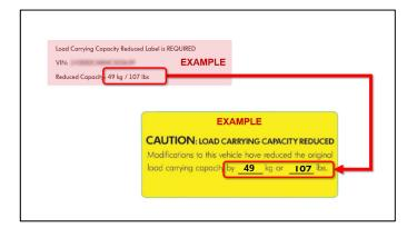
• Fill out the "Load Carrying Capacity Reduced Label" and apply it on the B-pillar.
