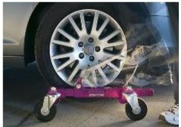
Figure 5 – Wheel Jack Dolly Installed
