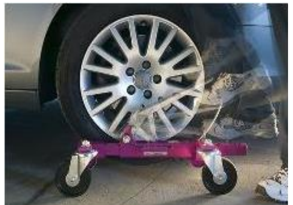
Figure 5 – Wheel Jack Dolly Installed
