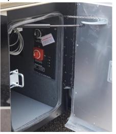
3. Using the 5/8" bit and the drill, remove the screws holding the DCD board in place. (The DCD board mounts in a black panel that has a flange which is held in place.
