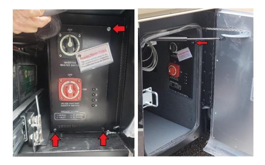
4. Remove the DCD panel, and check and adjust the torque as necessary.
