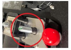
7. Examine the rear side of the inverter rotary knob for any signs of overheating or damage.
