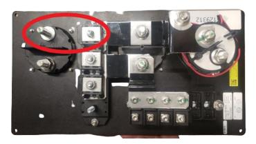
9. Using the cable provided, connect one end of the cable to the stud for the inverter switch. This will require using the torque wrench set on 100 in lbs.
