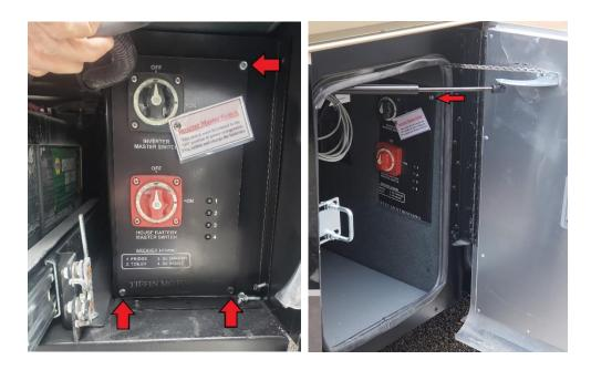
4. Remove the DCD panel, and locate the buss bar between the inverter stud and the 400A Zcase fuse.
