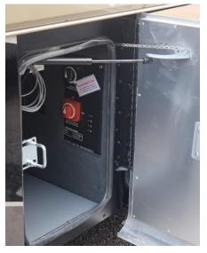
3. Using the 5/8" bit and the drill, remove the screws holding the DCD board in place. (The DCD board mounts in a black panel that has a flange which is held in place.
