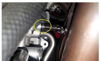
To ease access to the oil pipe plate bolt for the engine side of the oil cooler outlet pipe, use a 1/4 inch socket extension with a U-joint socket adapter in the gap between the top of the oil cooler and the bottom of the radiator, between the #2 and #3 exhaust pipes.
