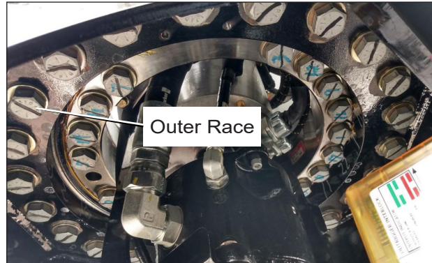
Figure 2 — Outer Race Rotation Bearing Cap Screws and Washers
