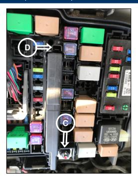
4. Install the new multi-fuse, placing the junction cable over the multi-fuse mounting tab, and the retaining washer on top. Torque to specification.
