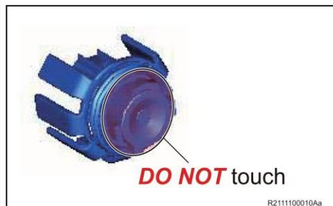
**DO NOT touch the printed circuit board of the removed back-up light LED, since static electricity may damage the LED.**
