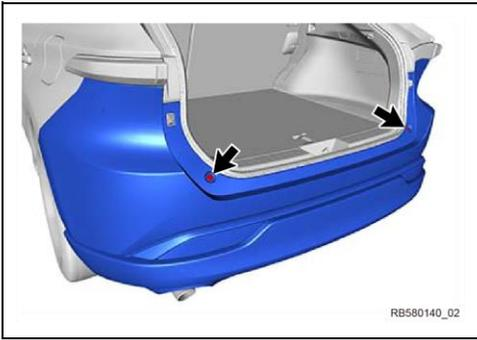
e. Install the 2 rear bumper stoppers (screw and grommet).
