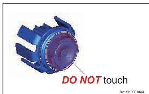
**DO NOT touch the printed circuit board of the removed back-up light LED, since static electricity may damage the LED.**
