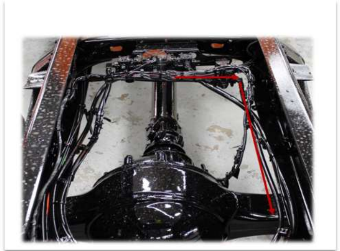
Air Brake Hose Is Not Exposed To Potential Damage
