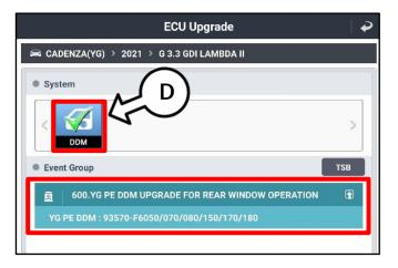
8. The ECU upgrade will begin and the progress of the upgrade will appear on the bar graph. Upgrade part (1/2) (E) will download the upgrade event to the VCI-II. Upgrade part (2/2) (F) will upgrade the ECU.
